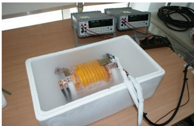
Fig. 2. Photo of a superconducting fault current limiter during a short circuit test [4]
