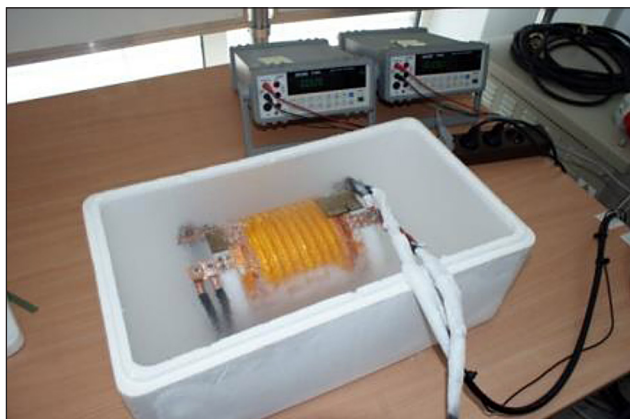
Fig. 2. Photo of a superconducting fault current limiter during a short circuit test [4]
